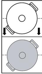
The cookware is detected and the previously selected power level and  $\text{t}$  flash alternately on the display for the new cooking zone.
