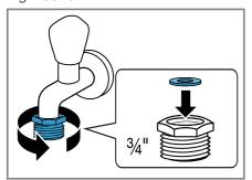
4. Open the water tap carefully and check that the connection points are tight.
