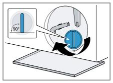
The handle on the pump cap must be in a vertical position.
