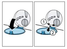
**5.** Slide a sufficiently large container under the opening.
