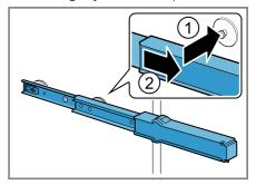
2. Place the telescopic rail on the rear pin 1 and push the locking mechanism back 2.
