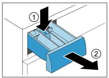
3. Pull out the insert upwards.
