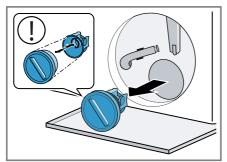
Clean the interior, the thread on the pump cap and the pump housing.
