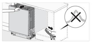
• Check that the machine is installed such that the door opens freely, otherwise door lock functionality may be disrupted.
