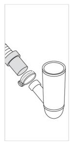
The drainage hose can also be connected to a connection nipple on the sink unit's water trap. The connection nipple must have an internal diameter of at least 14 mm.
