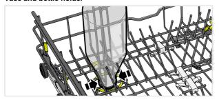
Install the vase and bottle holder above the left spray nozzle. (Found in the enclosed plastic bag.)
