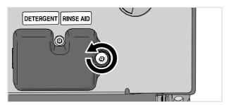
2. Connect the external cables for detergent to the auto dose connector.
