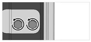
2. Attach the nipple and connect the hose for detergent.
