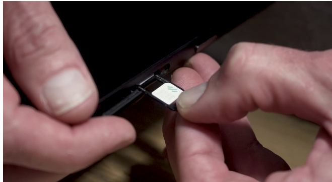
Fig 1. SIM/SD Door on side of Cat S75 handset
