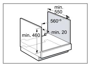
The worktop must be secured to the fitted unit.
