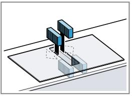
6. Insert the grease filter.
