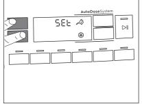
4. Touch related tank buttons to toggle function off and on. The display shows OFF when a tank is disabled or shows tank indicator when it is enabled.
