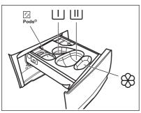
C - Compartment for detergent pods (Max 2 pods). When using detergent tablets, make sure that the Pods option is activated.
