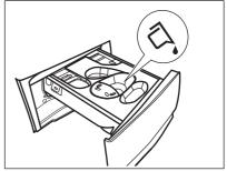
**c)** Put the **tablets** in the compartment . Make sure that the Pods option is activated.
