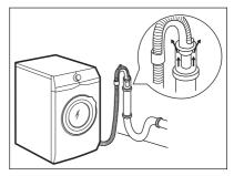
**1** The end of the drain hose must always be ventilated , i.e. the inner diameter of the drain pipe (min. 38 mm min. 1.5") must be larger than the external diameter of the drain hose.
