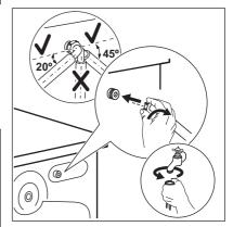
2. Position it toward left or right depending on the positon of the water tap. Make sure that the inlet hose is not in vertical position.
