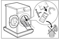
Accessories delivered with the appliance may vary depending on the model. 2. Put the packaging element on the floor behind the appliance and carefully put it down onto its rear side. Remove the polystyrene protection from the bottom.
