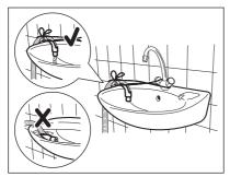
**ì** Make sure that the plastic guide cannot move when the appliance drains and the drain hose end is not immersed in the water. There may be a return of dirty water into the appliance. 3. If the end of the drain hose looks like this (see the picture), you can push it directly into the stand pipe.
