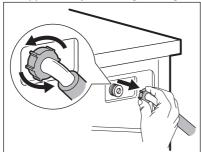
Clean the valve filter on the back of the appliance with a toothbrush.
