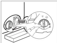
Turn the filter 180 degrees in anticlockwise direction to open it, without removing. Let the water flow out.
