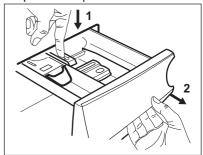
Remove the top part of the additive compartment to aid cleaning and flush it out under running warm water, to remove any traces of accumulated detergent. After cleaning, replace the top part in its position.
