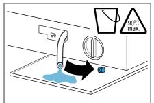
8. Firmly press on the sealing cap.
