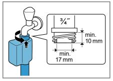
2. When connecting to a 21 mm = 1/2" tap, first fit the adapter with a sealing washer.
