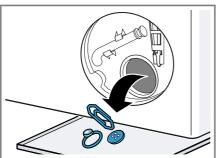
**3.** Make sure that the impeller in the drain pump can be rotated.
