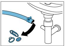
**5.** Reattach the water outlet hose and secure the connection point using the hose clamp.
