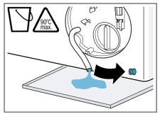
9. Firmly press on the sealing cap.
