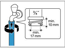
When connecting to a 21 mm = <sup>1</sup>/<sub>2</sub>" tap, first fit the adapter with a sealing washer.
