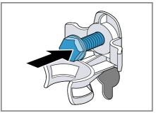
Insert the power cord into the holder ① and tighten all four screws for the transit bolts with a WAF 13 wrench ②.
