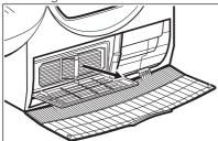
**6.** Clean the condenser in vertical position over a basin. Rinse through with a hand shower.
