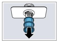
**4.** Press the locking catches ① together and lift the coarse filter out (2)
