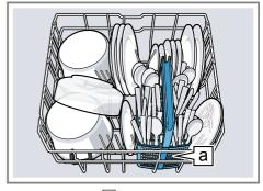
Cutlery basket a1 Large plates up to a diameter of 31/34 cm<sup>1</sup> can be arranged as shown.
