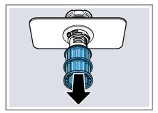
4. Press the locking catches 10 together and lift the coarse filter out 2.
