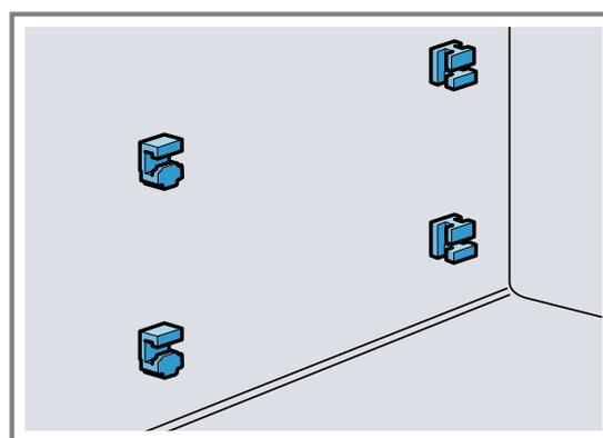
1. Hook the front retainers with the hook into the round hole at the top and set them at a slight angle **1**.
