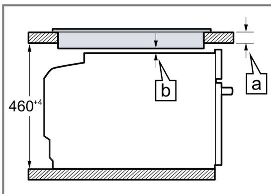
The minimum worktop thickness **[b]** a is based on the required minimum clearance **[a]**.
