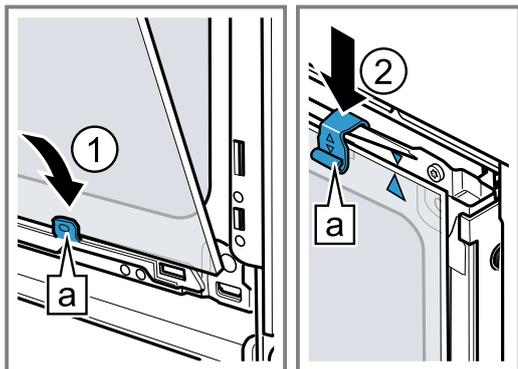
4. Attach the front pane downwards into the left- and right-hand retainers **a** **1**.
