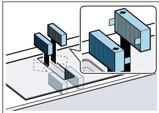
6. Insert the grease filter.
