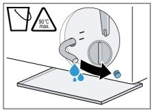
8. Firmly press on the sealing cap.
