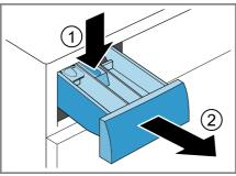
3. Pull out the insert upwards.
