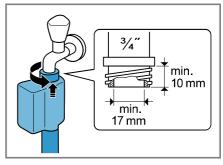
When connecting to a 21 mm = 1/2" tap, first fit the adapter with a sealing washer.
