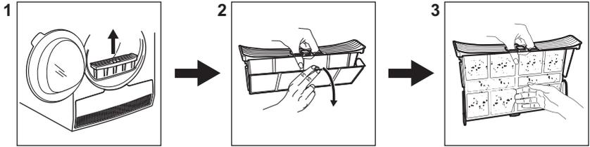
At the end of each cycle the filter symbol
