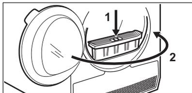
1) If necessary remove fluff from the filter socket and gasket. You can use a vacuum cleaner.
