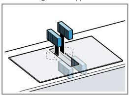
6. Insert the grease filter.
